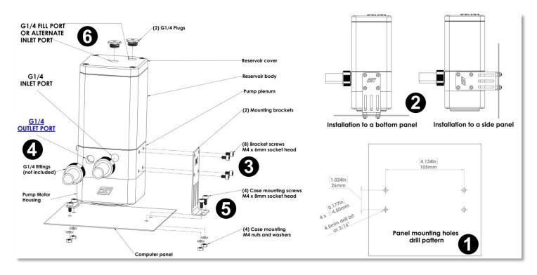
Preliminary note of caution! <u>Never use excessive torque to lock the screws or the fittings</u>. Excessive torque will result in damage to your product, and is not covered by our warranty. The rule of thumb is to NOT exceed ¼ of a turn past mating point of the parts.
